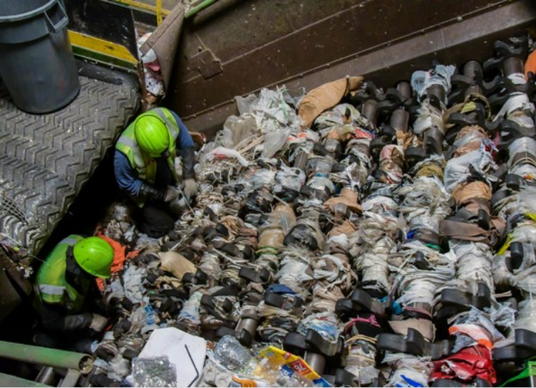
Workers removing tangled plastic bags from equipment.
