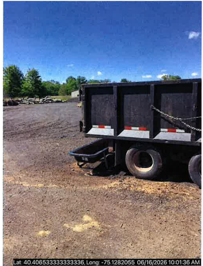
Photo #4 Trailer holding FPR with trough for draining into underground storage tank.
